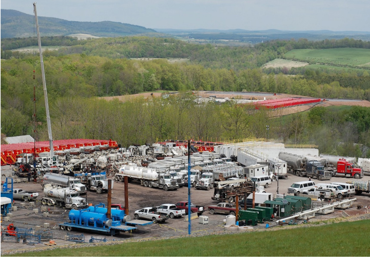
Figure 3-11. Well site with equipment (and pits in the background) in preparation for hydraulic fracturing in Troy, Pennsylvania.
