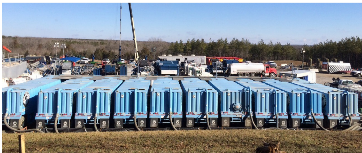
Figure 3-13. Water tanks (blue, foreground) lined up for hydraulic fracturing at a well site in central Arkansas.
