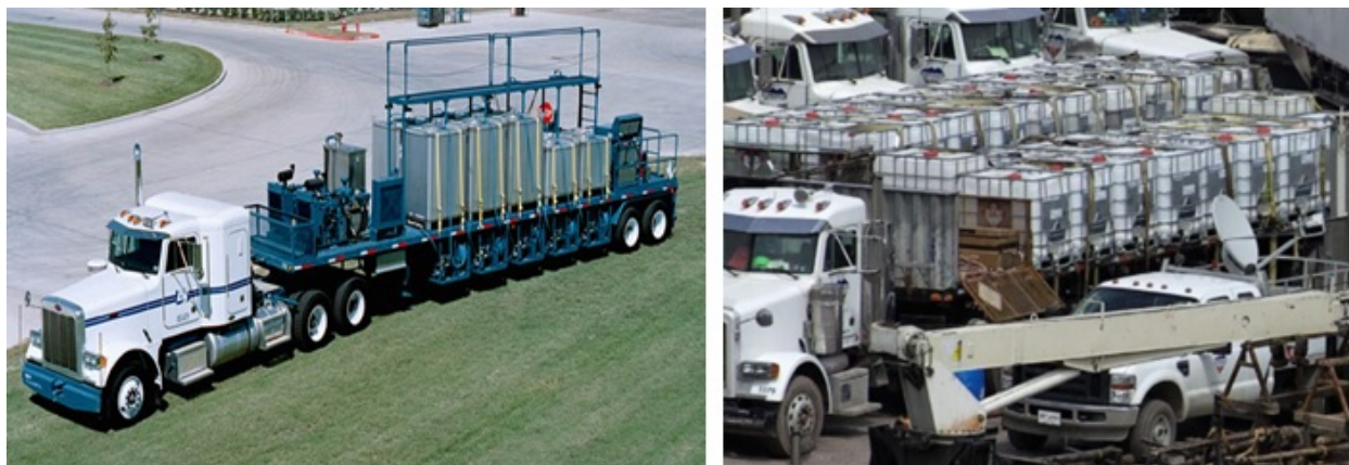
Figure 5-7. Metal and high-density polyethylene (HDPE) additive units.
