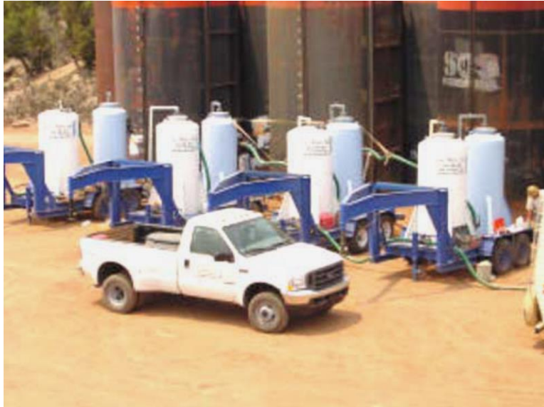
Figure F-3. Picture of mobile electrodesalination units in Wyoming.
