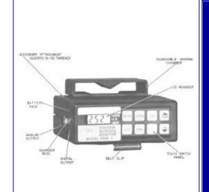
The MINIRAM (Miniature Real-Time Aerosol Monitor) Model PDM-3 is an ultra-compact personal size airborne particulate monitor. The MINIRAM can be used to measure the concentration of all forms of aerosol: dusts, fumes, smokes, fogs, etc. It's small size and weight, and concentration-averaging features permits its use as a personal exposure monitor.
